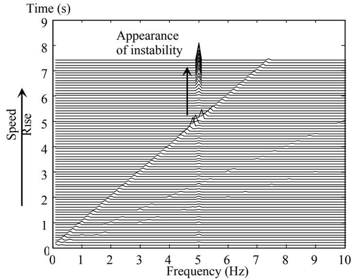
**Figure 4.** *Frequency spectrum upon starting of a rotating system. Measurement with accelerometer secured to casing. Instability appearance*
