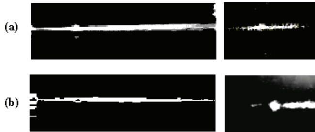
Figure 3.23. Photograph of light propagation of (a) planar and (b) channel YCOB \text{He}^+ -implanted waveguide([Vin 2004])
