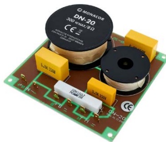
Figure 2.20. A two-way crossover (Monacor DN-20)
