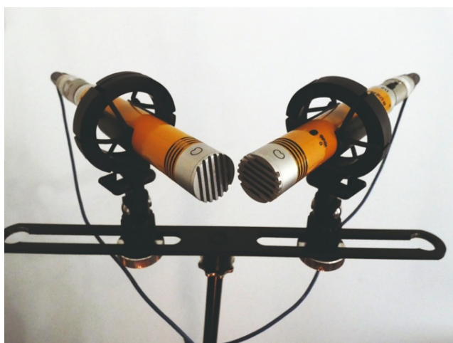
Figure A4.13. A Blumlein installation (source: www.musicradar.com )
