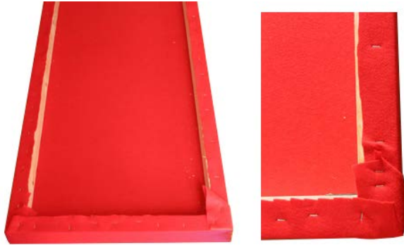
Figure 3.14. Back of frame with stapled fabric
