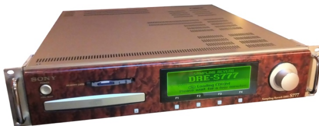
Figure 1.9. The first convolution reverb, Sony DRE-S777
