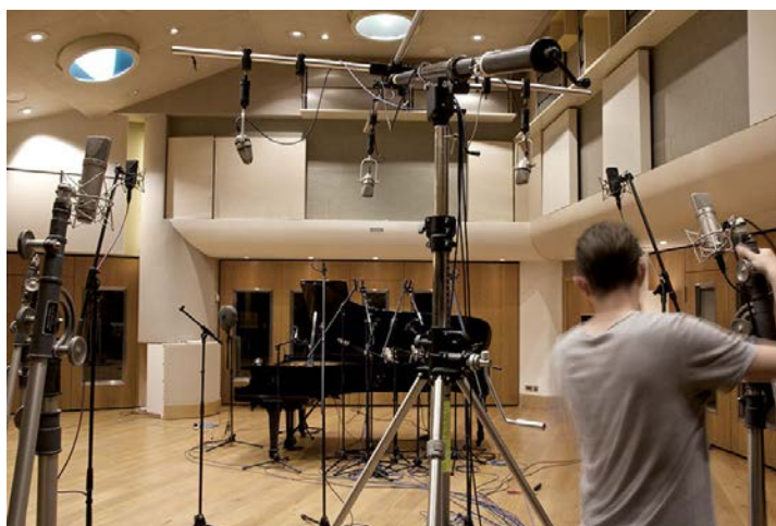
Figure A4.11. Decca tree installation (source: www.musictech.net )
