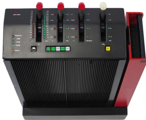
Figure 1.8. The first EMT 250 digital reverberator, dating from 1976
