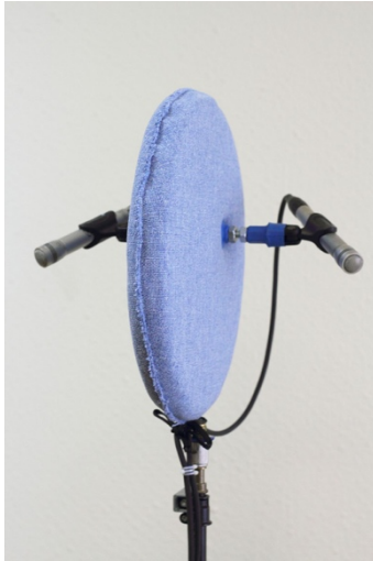
Figure A4.16. A Jecklin Disk installation (source: Wikipedia)
