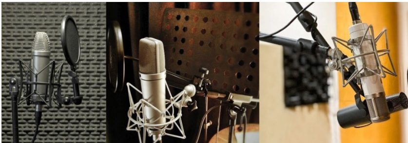
Figure 3.26. From left to right, stand microphone, boom microphone up, boom microphone down
