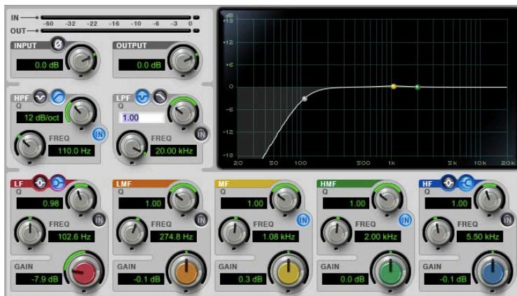
Figure 3.39. An HPF filter with the Avid Protocols seven-band equalization plugin
