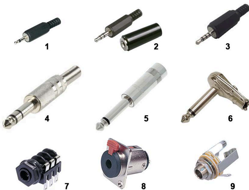
Figure A2.1. Some models of coaxial jacks. 1) subminiature 2.5 mm mono male jack, 2) 3.5 mm miniature stereo male jack, 3) 3.5 mm miniature multi-pole male jack, 4) 6.35 mm (1/4") stereo male jack, 5) 6.35 mm mono male jack, 6) 6.35 mm angled mono male jack, 7) 6.35 mm chassis stereo jack, 8) 6.35 mm chassis mono jack, 9) 6.35 mm chassis mono jack
