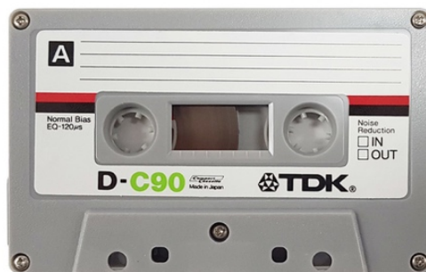
Figure 1.29. A type I – C90 (2 X 45 min) mini-cassette from TDK
