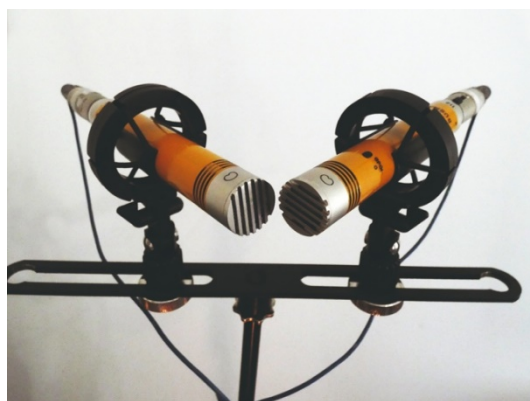
Figure A5.13. A Blumlein installation (source: www.musicradar.com )
