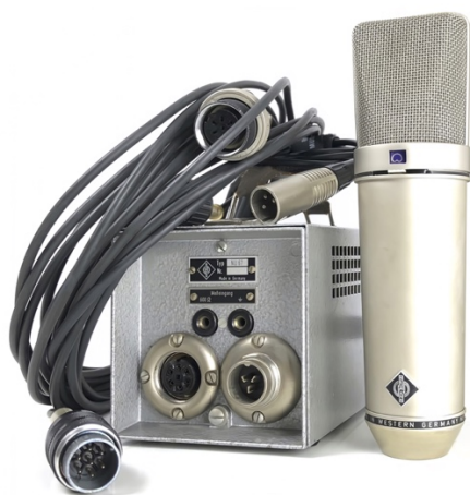
Figure I.3. The famous Neumann U67 tube microphone and its power supply
