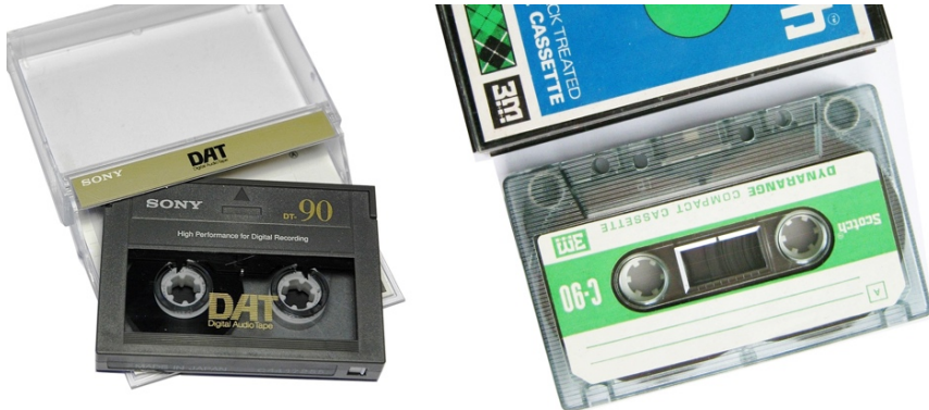
Figure 1.41. A DAT cassette (73 x 54 10.5 mm), on the left, compared to a mini-cassette (100 x 83 x 12 mm), on the right
