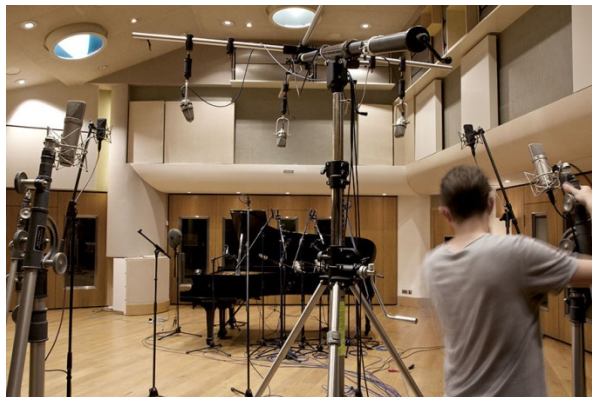
Figure A5.11. Decca tree installation (source: www.musictech.net )
