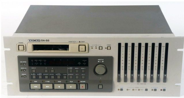
Figure 1.46. The Tascam DA-88 digital player-recorder
