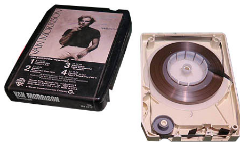
Figure 1.23. An 8-track tape and its internal structure
