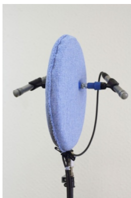
Figure A5.16. A Jecklin Disk installation (source: Wikipedia )
