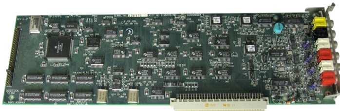
Figure 1.54. The Audiomecia II board in Nubus format for Apple Macintosh
