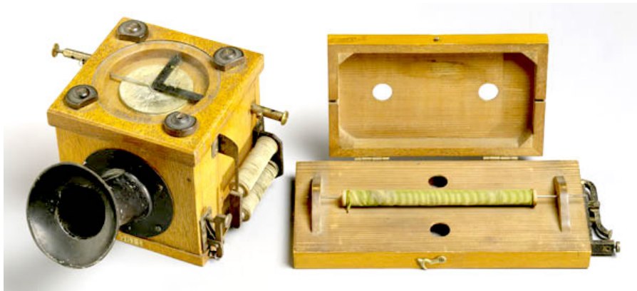
Figure 3.3. Reis's telephone with its transmitter (microphone), left, and receiver, right (source: Deutsches museum)
