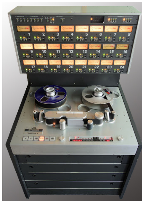
Figure 1.34. A 24-track 2-inch multitrack (Studer A800 – MKII), a standard of excellence in the studios of the 1970s and 1980s
