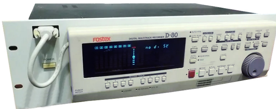
Figure 1.49. The Fostex D80 hard disk recorder – 8 tracks (1996)
