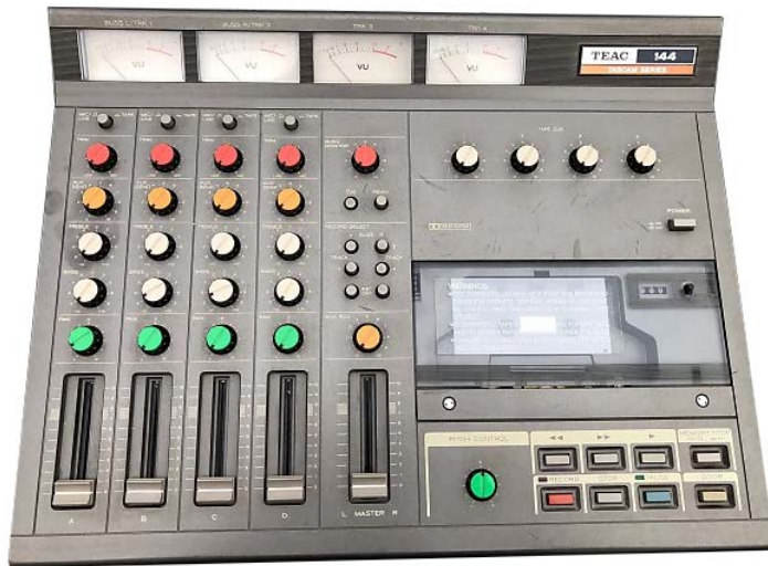
Figure 1.31. The Portastudio 144 stand-alone multitrack from Tascam (1979)
