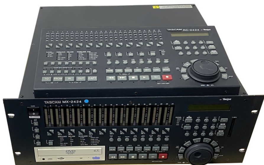
Figure 1.50. Tascam MX-2424 – 24-bit, 96 kHz, 24-track hard disk recorder (2004) with its RC2424 remote control
