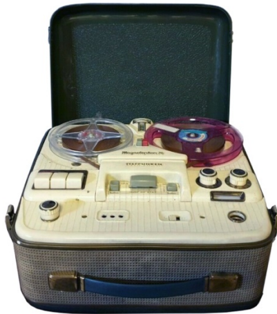
Figure 1.26. The Telefunken 76 (Tube) tape recorder, 4 tracks (stereo 2 X 2 tracks), speed: 4.75–9.5 cm/s, reel to 15 cm diameter, dating back to 1960
