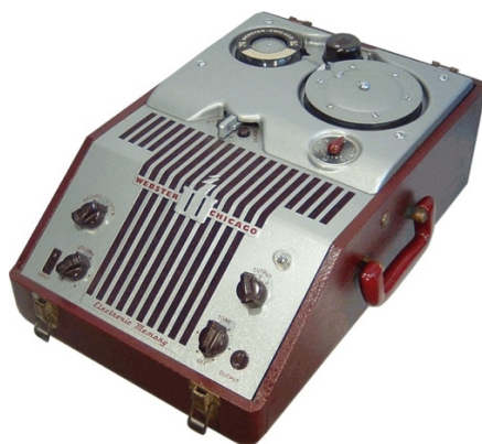
Figure I.2. A wire recorder, the Webster Chicago 180-1 (1949)
