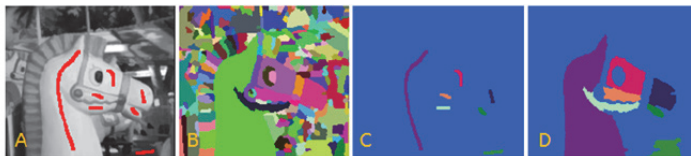
Figure 14.15. Segmenting marked regions. a) Initial image on which markers have been superimposed. b) The partition resulting from the segmentation. c) The markers have been labeled. d) All regions of the partition touched by a marker get the label of this marker
