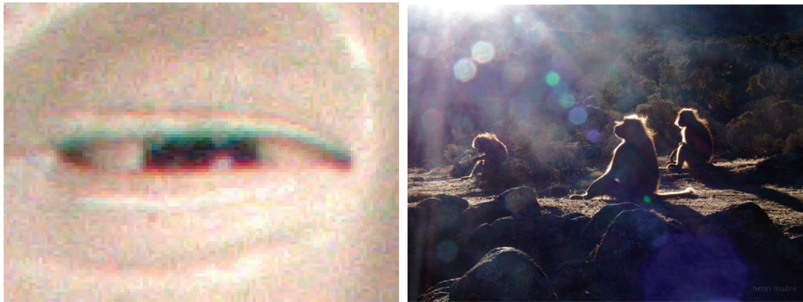
Figure 2.30. On the left, chromatic aberrations. The red or blue edging that affects the contours above and below the eye can clearly be seen (the full image where this detail is taken from is in Figure 8.2). Right image: multiple reflections on the various lenses of the objective: the heptagonal shape of these reflections comes from the diaphragm composed of seven plates opening like a hand fan. The shape of the diaphragm is involved in these reflections, but also in the shape of the blurring of the objects that are focused
