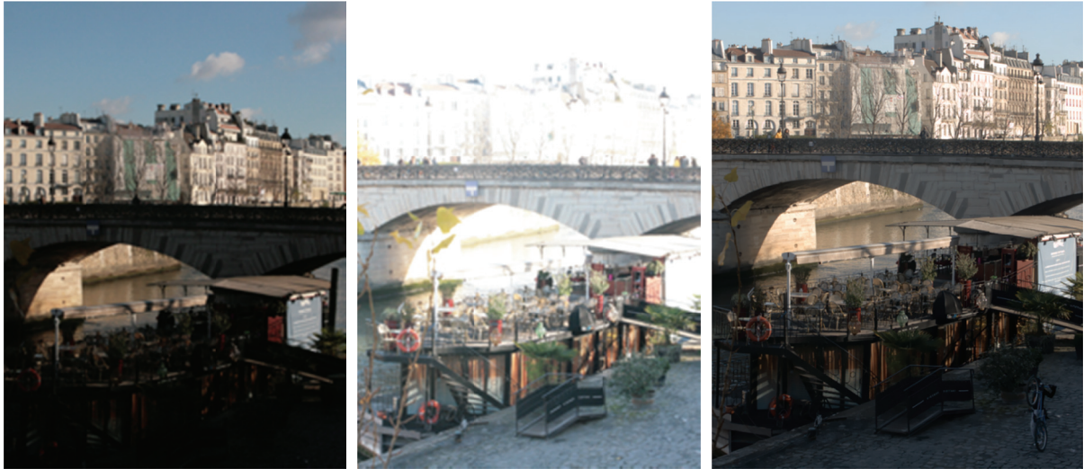
Figure 10.10. HDR treatment of four images (only the two extreme images are presented, with the least exposed on the left and the most saturated in the center). The result of this treatment, for the shared zone of the images, accounting for movement and compressed onto 8 bits, is shown on the right. Taken from [AGU 14a]
