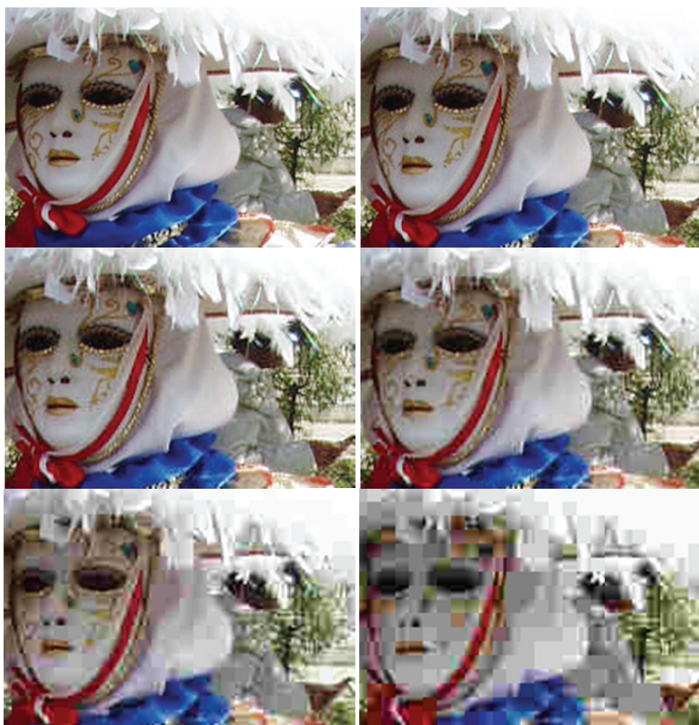
Figure 8.5. Magnification of an area of an image encoded using JPEG. The top left image is the non-encoded original. The whole image has then been compressed by factors of 5.4 (top right), 12.1 and 20 (central line), and 30 and 40 (bottom line)
