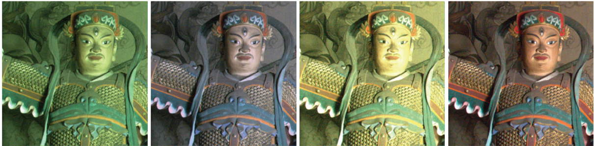
Figure 5.9. White balance. From left to right: original image, whose parameters (illuminants, camera settings) are unknown, as recorded on chip (during viewing the primaries are assumed to be those of the sRGB space); white balance by the von Kries model, under the gray-world hypothesis, then under the white-page hypothesis, finally on the right, correction made with the (unknown) algorithm of the camera. The very wide variety of renderings can be observed in this difficult situation where the light sources are artificial and the colors strong
