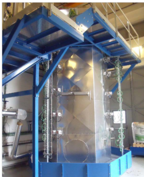
Figure 8.17. Pilot PCM storage by CEA-Liten (Garcia et al. 2015)
