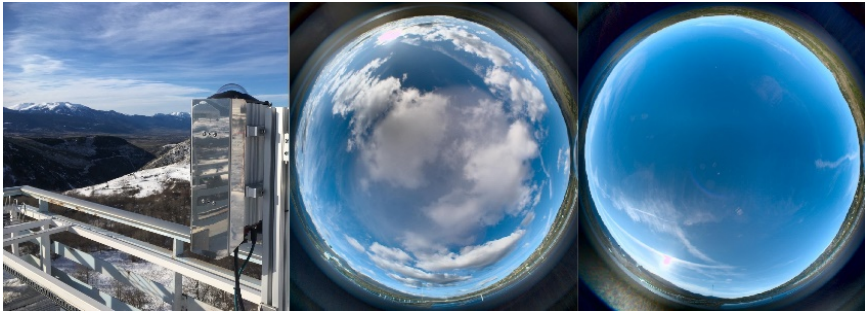
Figure 2.17. The PROMES sky imager installed at Odeillo and several HDR images acquired (after tone correspondence)
