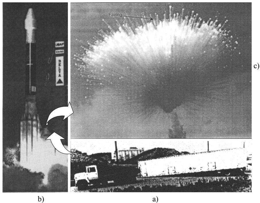
**Figure 1.10.** Delta II mission 241 explosion, from [GUN 99], a catastrophic failure which could have been avoided by pre-usage health monitoring – a) road transportation: the rocket is inside the trailer, here detached; b) Delta II liftoff; c) the explosion, initiated from a crack in one of the graphite epoxy motors situated at the base of the rocket
