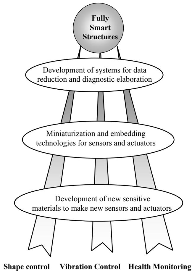
**Figure 1.7.** Common basis and complementarity of SHM, shape control and vibration control
