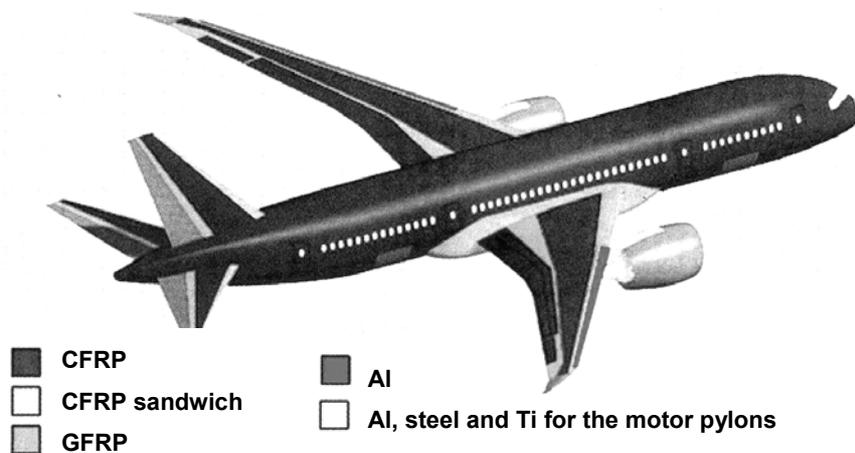
**Figure 1.6.** Example of the increasing importance of composites in civil aircraft: the 7E7 Dreamliner has 50% of its structure made of composites. For this aircraft, impact detection monitoring systems are envisaged for outer panels
