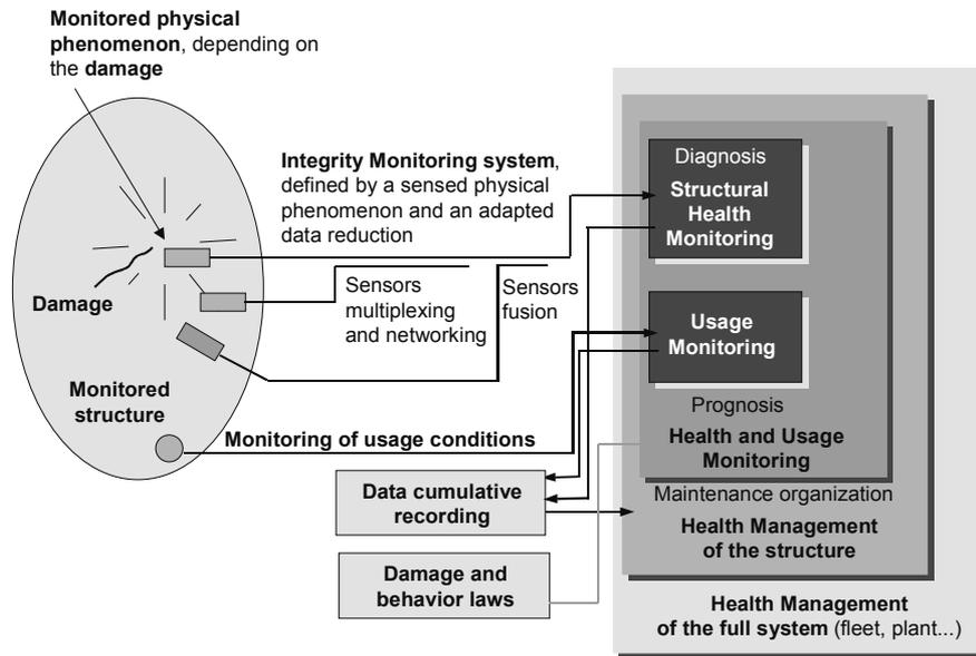
**Figure 1.1.** Principle and organization of a SHM system
