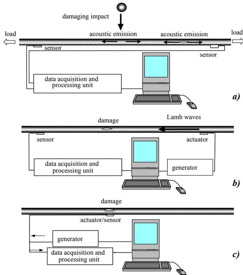
**Figure 1.13.** Flexibility of monitoring techniques using piezoelectric patches: a) passive method: acoustic emission technique, b) active method: acousto-ultrasonic technique with generation of Lamb waves, c) active method: electromechanical impedance technique
