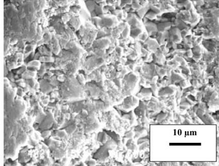
**Figure 3.7.** Alumina surface showing significant wear of the material characterized by grain pull-out
