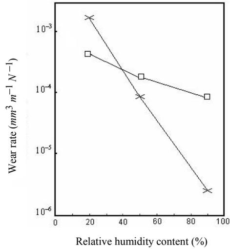
**Figure 3.8.** Variations in the rate of wear of  $\text{Al}_2\text{O}_3/\text{Al}_2\text{O}_3$  (□) and  $\text{Si/SiC}$  (×) couples/pairs as a function of residual humidity. Tests were carried out with a reciprocating tribometer operating in the sphere/plane set-up and using a 5 mm diameter sphere under a normal applied load of 30 N. The sliding distance is 2 cm and the sliding speed is  $2 \text{ mm s}^{-1}$  [TAK 94b]
