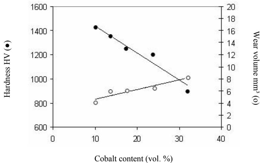
**Figure 3.11.** Variation of the hardness and volume wear of the WC-Co cermet as a function of the binding phase concentration. The tribometer used is of the pin-on-cylinder type and the applied load is 40 N [PAST 87]
