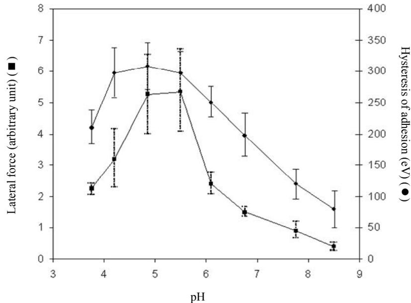
**Figure 2.29.** Lateral force (friction force) (■) and expended energy (hysteresis of adhesion) (●) measured with AFM/LFM at different levels of pH in a solution of 1 mM of NaCl between the silicon nitride tip of the AFM and a silicon oxide sample [MARTI 95]
