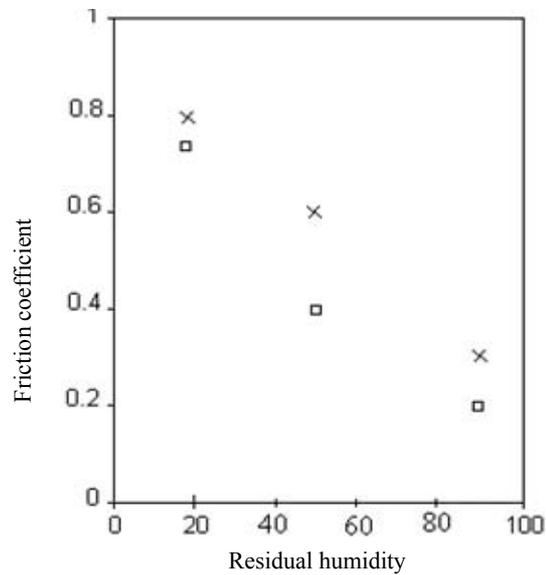
**Figure 3.9.** Variations of the friction coefficient as a function of residual humidity:  $\text{Al}_2\text{O}_3/\text{Al}_2\text{O}_3$  (×) and  $\text{SiC/SiC}$  (□) pairs (see Figure 3.8 for a description of the tests)
