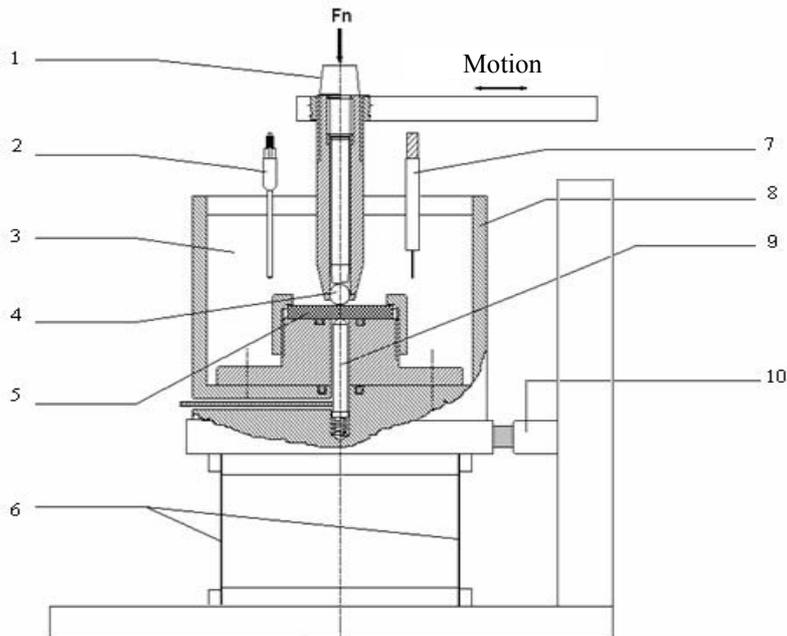
**Figure 2.40.** Tribocorrosion analysis set-up: 1) normal applied load; 2) reference electrode; 3) electrolyte; 4) ceramic sphere; 5) sample; 6) spring plates; 7) platinum counter-electrode; 8) PTFE electrochemical cell; 9) towards the potentiostat; 10) force sensor (adapted from [TAK 96])
