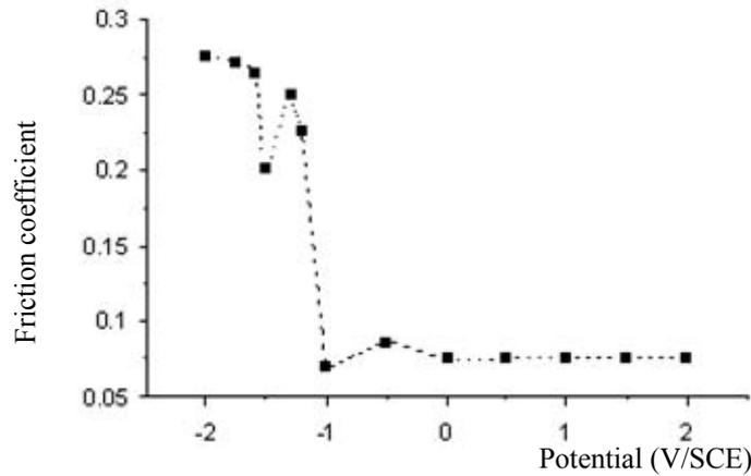
**Figure 2.44.** Variation of the friction coefficient of brass against a  $\text{SiO}_2$  sphere under a load of 9.8 N in a sodium laurylsulfonate solution with 0.1 M sodium sulfate. Values for the friction coefficient were recorded under several applied potentials [QIU 02]
