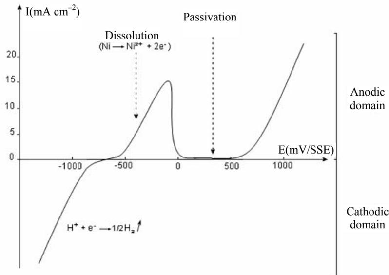
**Figure 2.41.** Polarization curve (intensity-contact potential) of nickel in a sulfuric environment ( $\text{H}_2\text{SO}_4$  1N); contact potentials are given relative to a saturated sulfate reference electrode (SSE)
