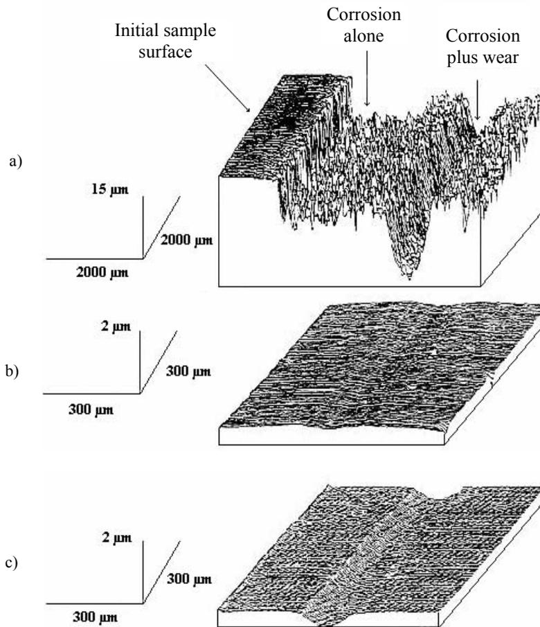
**Figure 2.42.** Surface states of nickel samples following a friction test in a  $\text{H}_2\text{SO}_4$  1N medium. The sample potential is: a)  $-350$  mV, b)  $500$  mV, c)  $-650$  mV (equally at  $-1300$  mV). The reference surface (Figure 2.42a) is the initial sample surface protected during the tribocorrosion test [TAK 97c]. Potentials were measured relative to a saturated sulfate electrode
