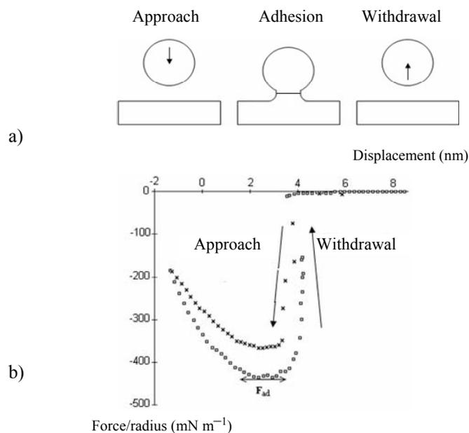
**Figure 2.26.** Forces of adhesion of a sphere on a plane. Forces curve obtained for two carbon surfaces with an SFA used in dry air: a) displacement of the sphere; b) force curves [GEO 00]
