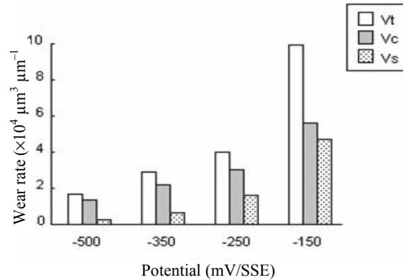
**Figure 2.43.** Volumes of material removed by tribocorrosion as a function of the applied potential imposed on nickel.  $V_w$ ,  $V_c$ ,  $V_s$  and  $V_t$  are the volumes defined in the text (see equation [2.45]). When measured in the cathodic domain, volume  $V_w$  ( $-1300$  mV) is  $130 \mu\text{m}^3 \mu\text{m}^{-1}$  [TAK 97c]
