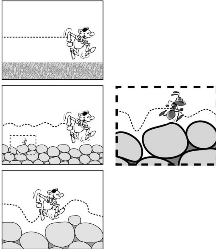
**Figure 3.1.** *The separation of scales is the sine qua non condition for a global description. Here it is only the case in the top picture: the property of homogenizability only has a meaning for the combination of the material and the phenomenon together (illustrations by Jacques Sardat)*
