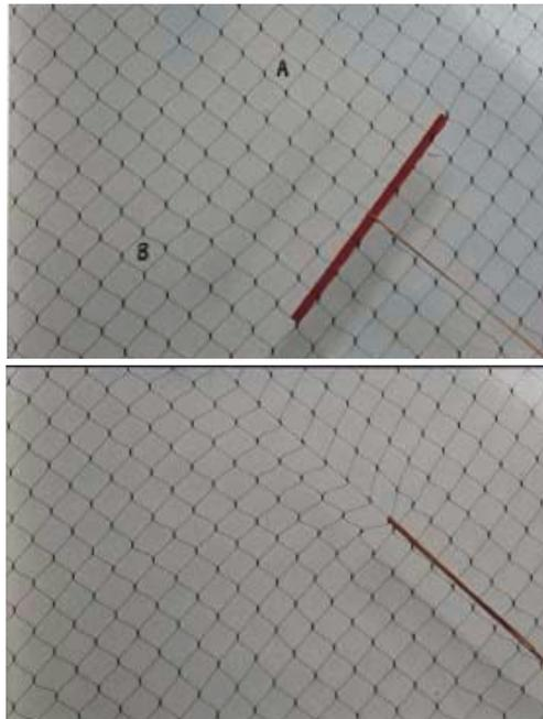
**Figure 3.4.** *Inhomogenous load: the quasi-periodicity relies on a separation of length scales: (a) a load which respects the separation of scales: the local quasi-periodicity is modulated by large-scale variations; (b) localized loading: the periodicity is lost along the line of the pull*
