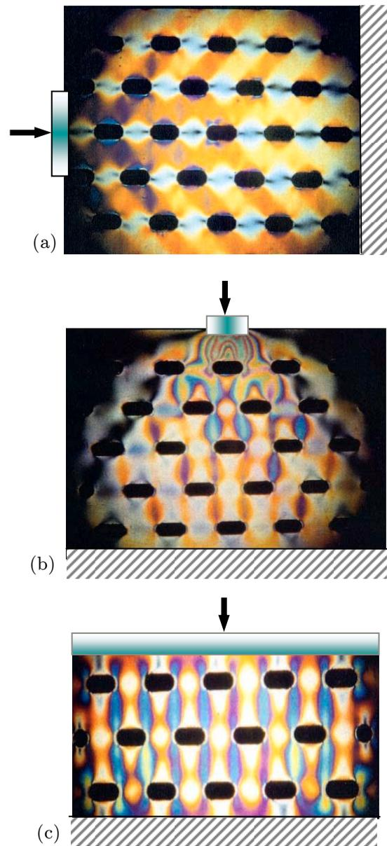
**Figure 3.6.** Role of the microstructure in the distribution of local and global forces: (a) inhomogeneous compression parallel and (b) perpendicular to the holes, (c) quasi-periodicity and edge effects under homogeneous compression for a plate which only consists of one-and-a-half periods
