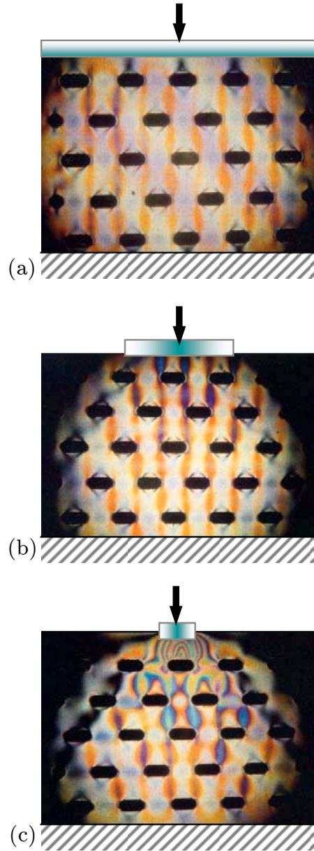
**Figure 3.5.** Condition of separation of scales, and quasi-periodicity of the fields in a periodic medium. Perforated plate subject to: (a) homogenous compression exerted by pressure across the width of the plate, (b) inhomogenous compression exerted by a pressure from above across a narrower width, (c) inhomogenous compression under point loading of the upper surface
