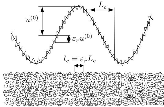
**Figure 3.11.** Estimate of the physical scale ratio  $\varepsilon_r$  for wave propagation:
