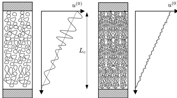
**Figure 3.9.** Estimate of the physical scale ratio  $\varepsilon_r$  in the case of simple compression:  $\varepsilon_r = \mathcal{O}(l_c/L_c)$
