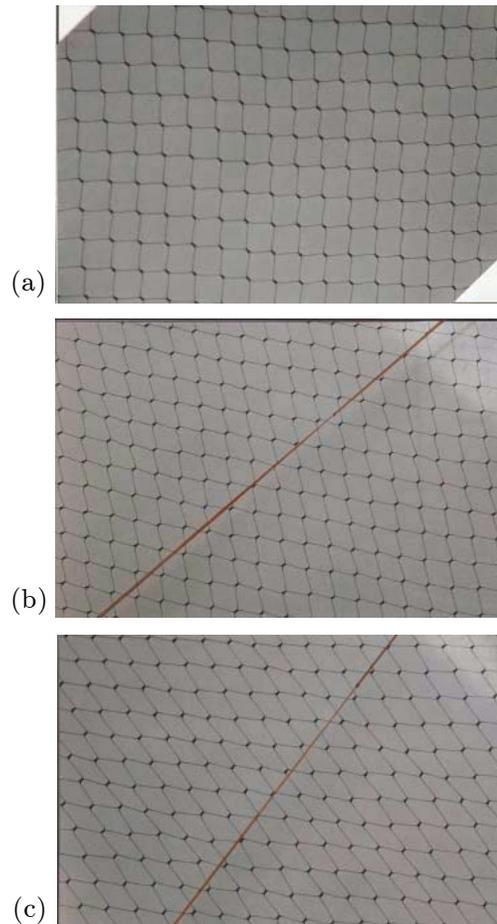
**Figure 3.3.** Visualization of a periodic net (a) of the periodicity under (b) moderate and (c) large deformations
