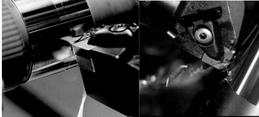
**Figure 1.1.** *Hard turning: cylindrical turning of hardened steel parts*
