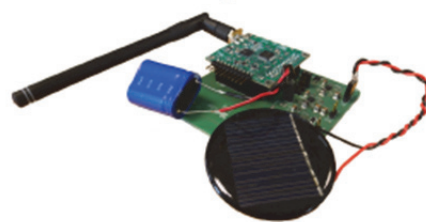
b) Prototype linking LoRa and multisource harvesting
