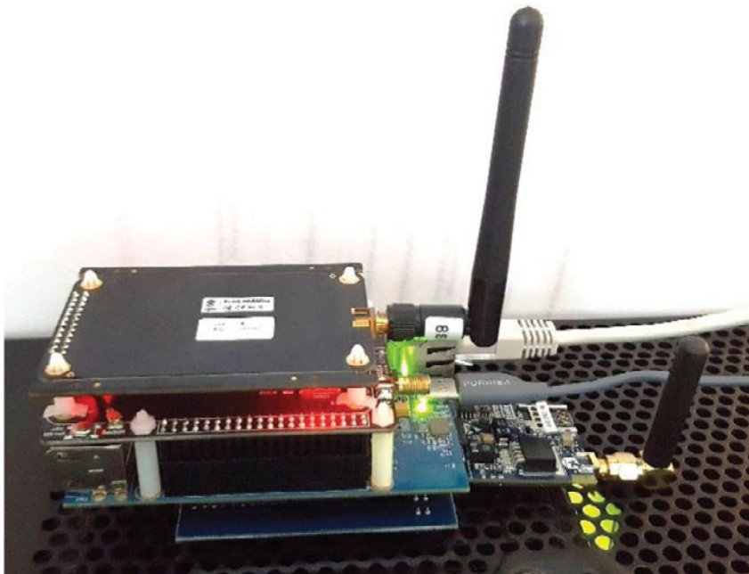
Figure 3.4. LoraWAN gateway using an RAK831 RF with a GPS (top two shields), the STM32MP1 and a 3G modem (bottom shield) when a wired connection is not available
